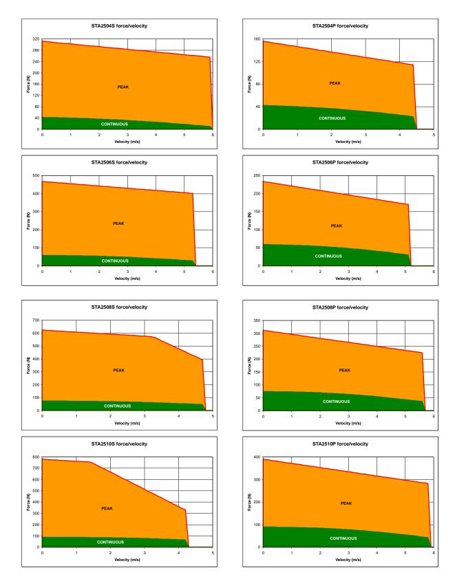
Figure C.6 - STA force / velocity profiles
