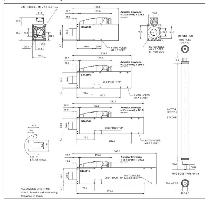
Figure 2.1- STA Outline drawings and mounting details
