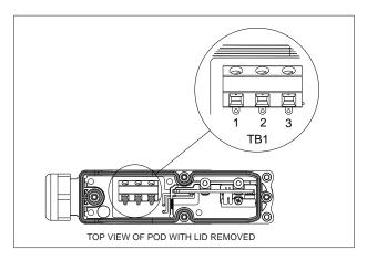
Figure C.4 - Power cable connection at TB1
