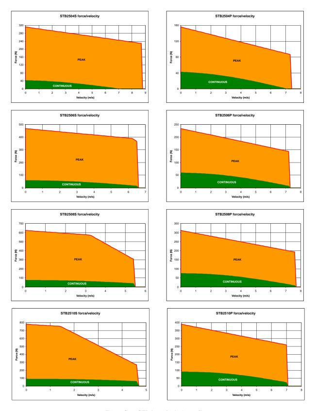
Figure C.7 - STB force / velocity profiles
